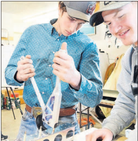
Kana Oliver for the Chieftain Aviation students from Joseph Charter School, Rylie Warnock and Gavin Baldwin, practice setting rivets on Micheal and Rene Flemmings's kit plane.
