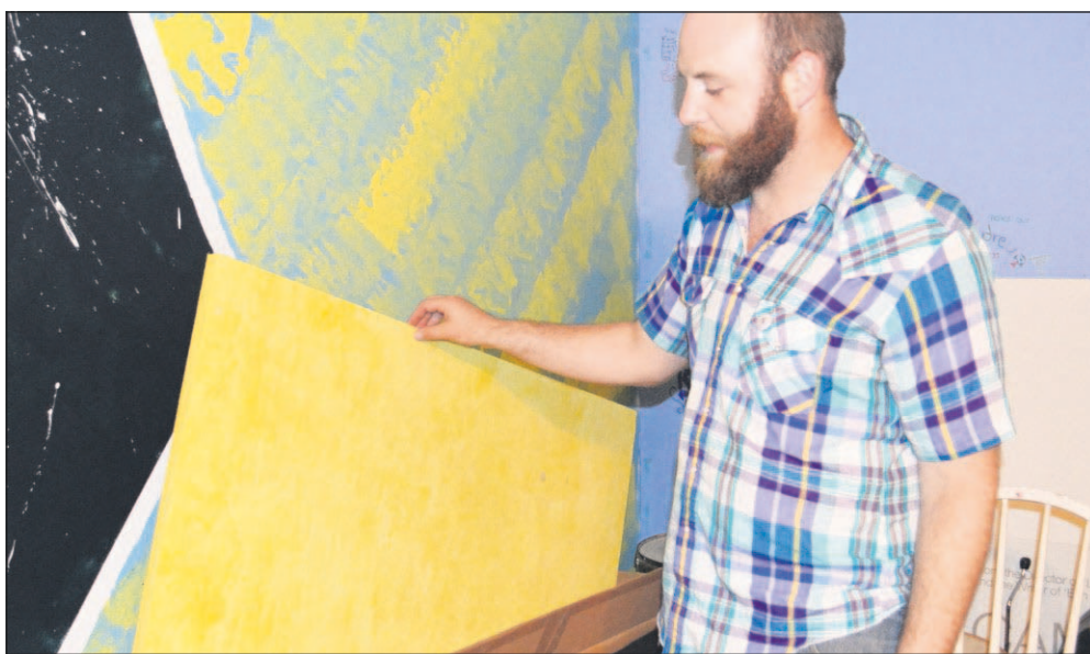
Sound recorder and musician Bart Budwig handles a 2 x 4 foot piece of OwensCorning fiberglass baffle material, excellent for muffling sound.
