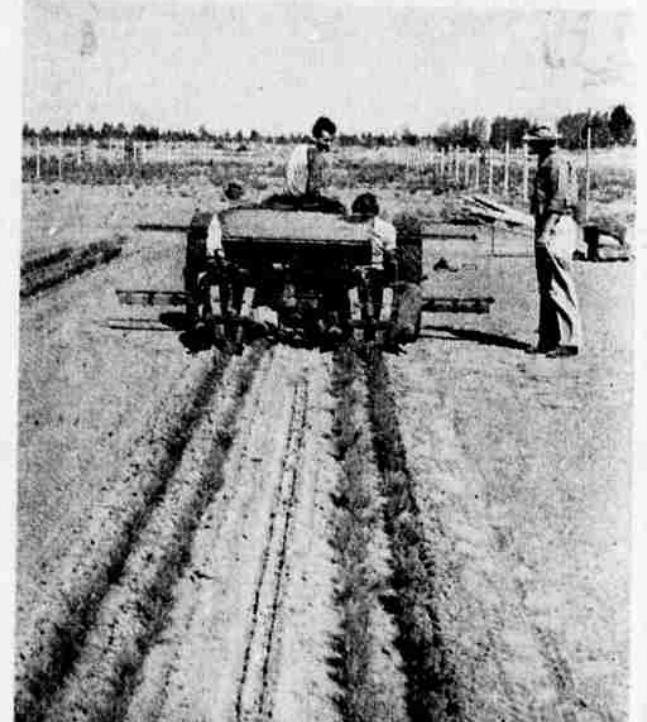
Transplanting equipment is shown here in operation. Four rows of seedlings are placed in the earth on each trip through the nursery field. Bob Blakley is looking back over the machine, to make certain all is well. Inspecting the work is Nurseryman Engstrom.
