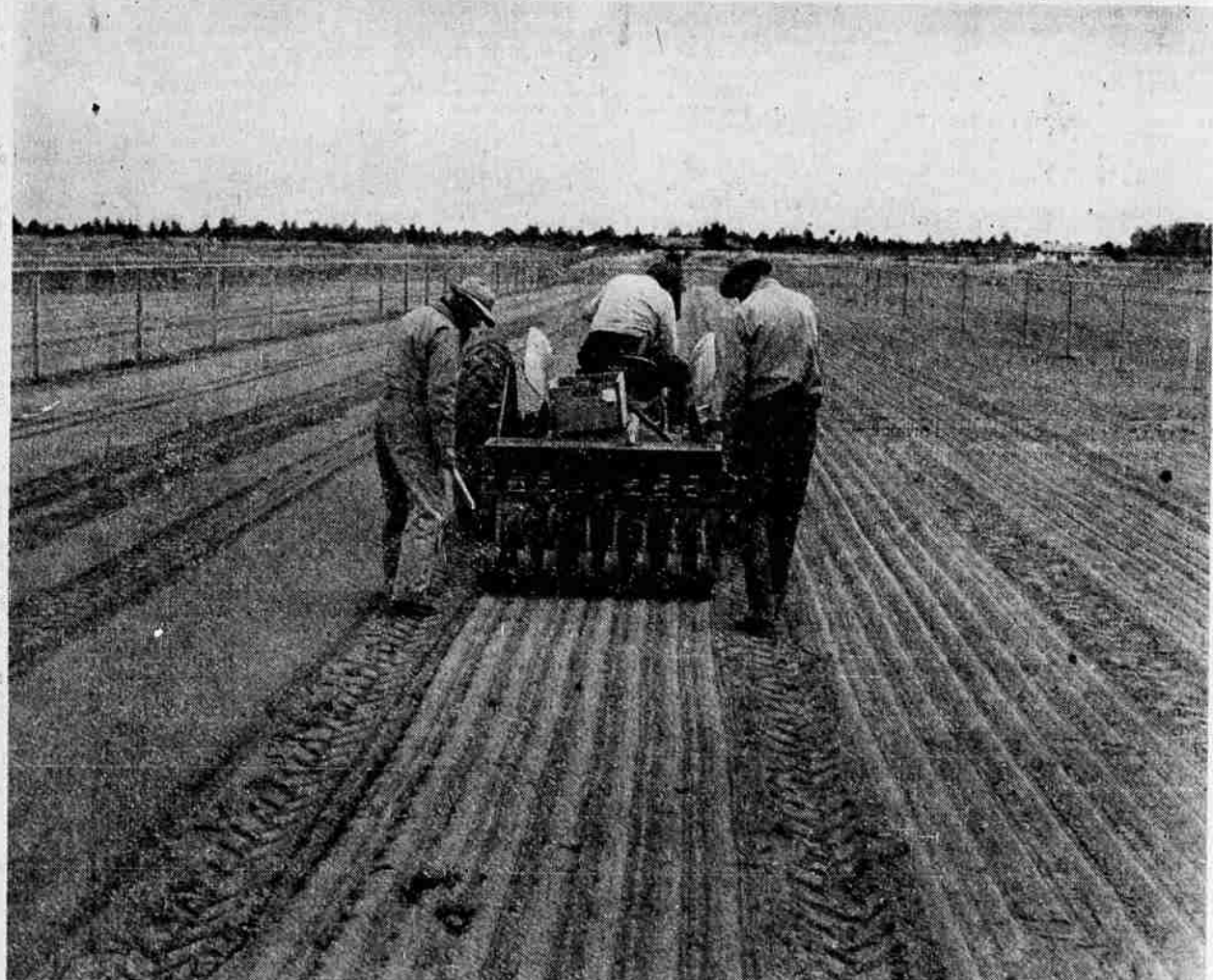
Carefully following long marked rows banked by sprinklers, a pine seed drill is shown in operation here, at the Bend pine nursery. Two men accompany the drill, to make certain the outlets are carefully feeding, and to be sure that the delicate seeds are covered. Just as soon as the seeds are in place, the overhead sprinkling system is placed in operation. Water sprays from each side of the tract, overlapping at the center.
