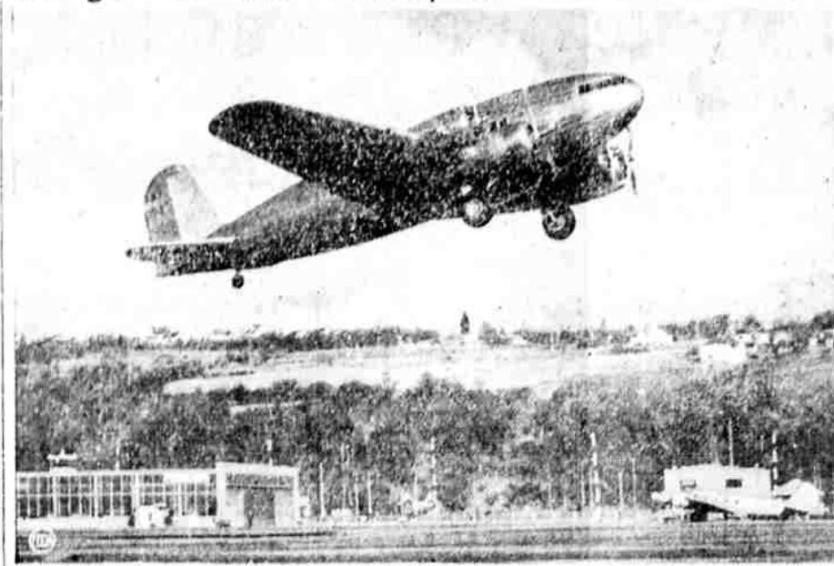
Under a full load of 22½ tons the new "Stratoliner" transport plane heads toward the clouds on a test flight at Seattle, Wash. Note the sharp angle of climb.
