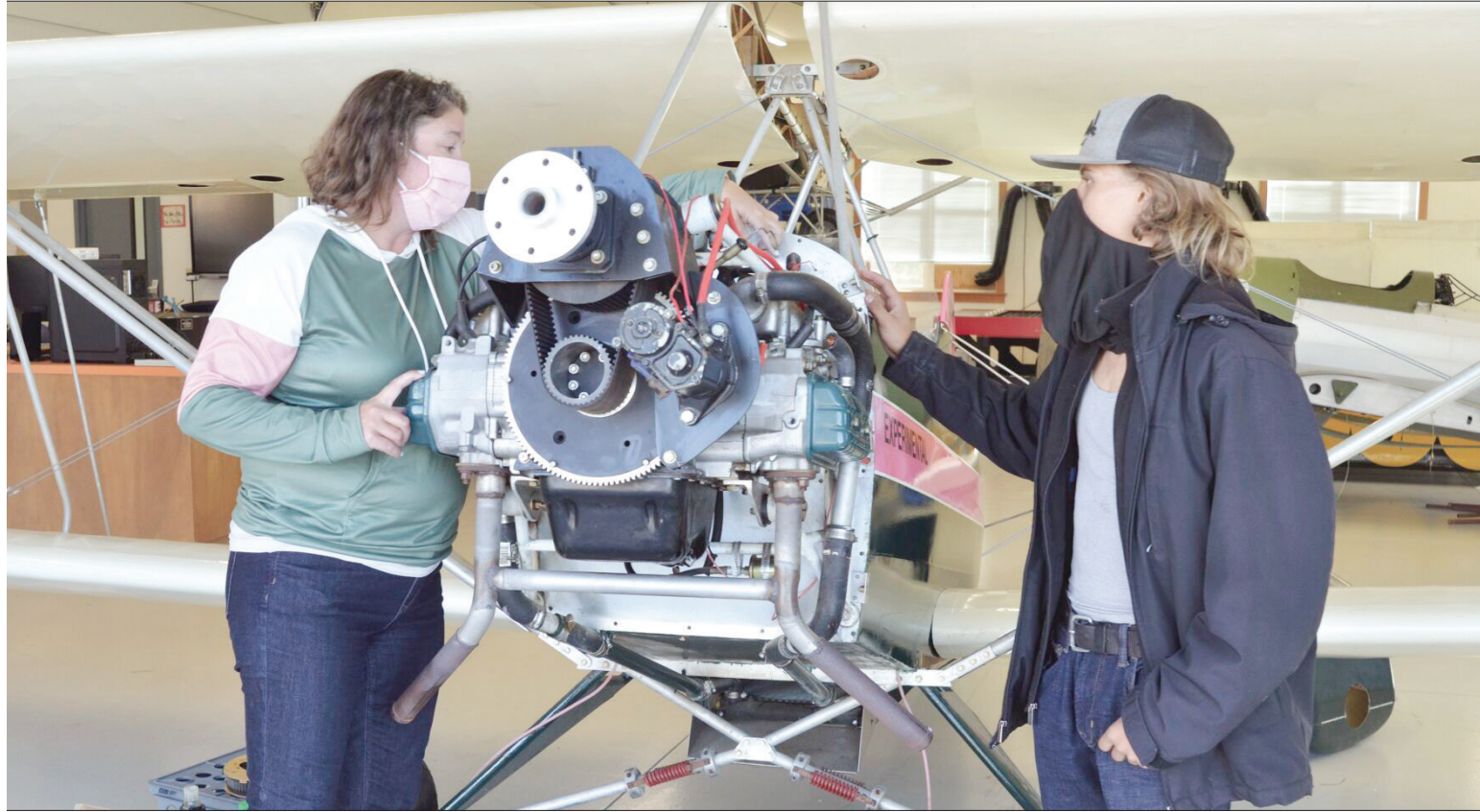
Lexi Rindfleisch, left, the new aviation instructor at Joseph Charter School, discusses a Subaru engine in an experimental aircraft with aviation student Jett Peterson on Thursday, Sept. 23, 2021.
