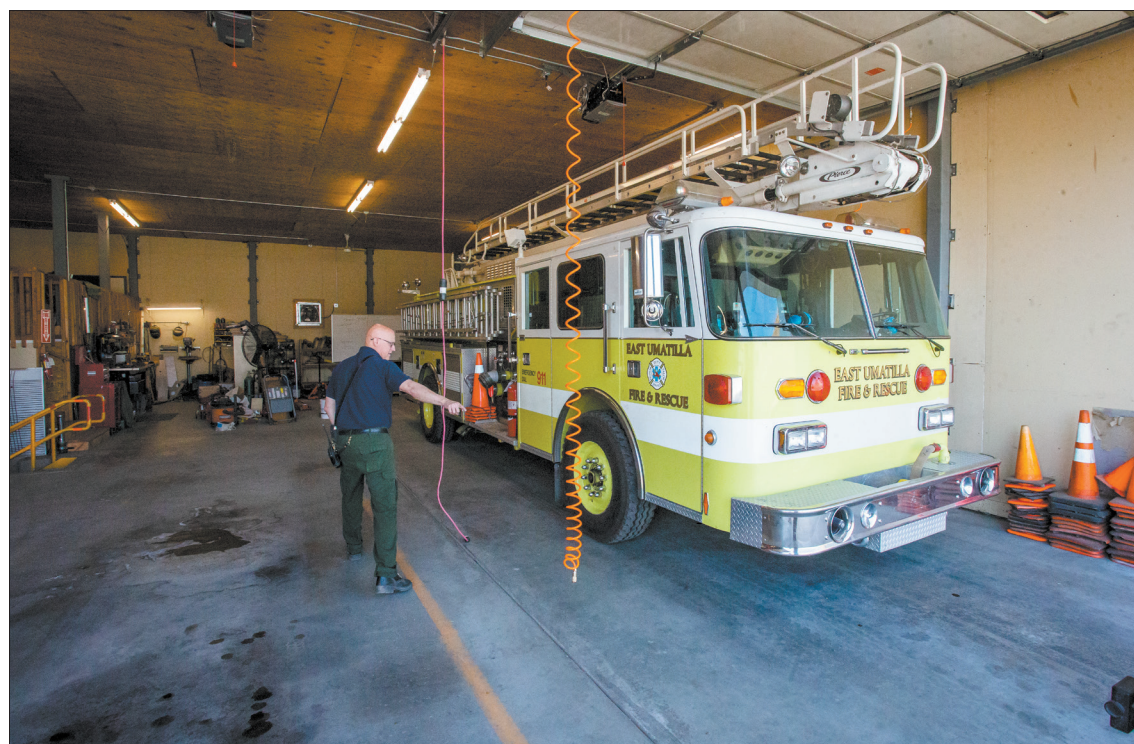
Ben Lonergan/East Oregonian East Umatilla Fire & Rescue Fire Chief David Baty explains issues with backing fire trucks into the district's Weston fire station on Wednesday, May 5, 2021. The primary issue is the steep angles of the driveway, which results in unnecessary stress and twisting on the vehicles' chassis and has caused vehicles to scrape the concrete if not backed perfectly.
