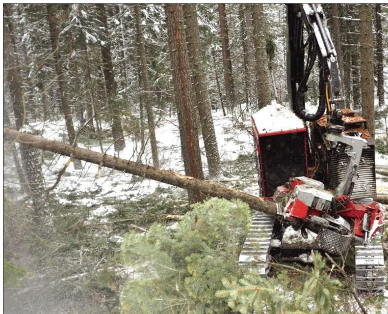
Bill Bradshaw/Wallowa County Chieftain A cut-to-length harvester operated by Tom Zacharias, of Pro Thinning Inc., of Joseph, falls, limbs and cuts a tree into standard 16-foot lengths in just minutes on Feb. 25, 2021, on the Lostine Corridor Public Safety Project.
