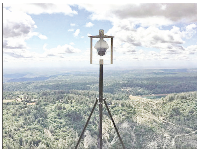
Oregon Department of Forestry Photo This close-up shows the high-definition, fire-detection camera mounted on a 110-foot tower atop Howard Butte that relays views showing smoke to the Central Oregon Interagency Dispatch Center in Prineville.
