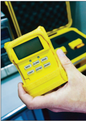
Staff photo by E.J. Harris Lt. Dennis McClure holds a personal radiation detector firefighters would wear when responding to a radiological incident.
