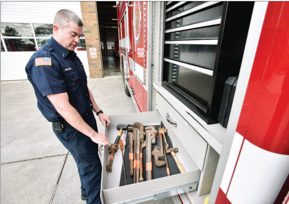
Staff photo by E.J. Harris Umatilla County Fire District 1 Lt. Dennis McClure opens a drawer with spark-free tools in it on the HazMat response vehicle.
