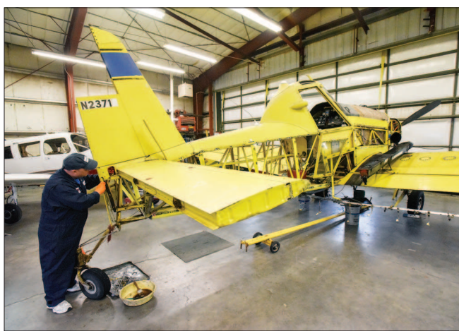
Staff photo by E.J. Harris Curtiss Nelson works on cleaning the tail structure of an Air Tractor while performing the annual inspection for the aircraft Thursday at Pendleton Aircraft Service at the Eastern Oregon Regional Airport in Pendleton.
