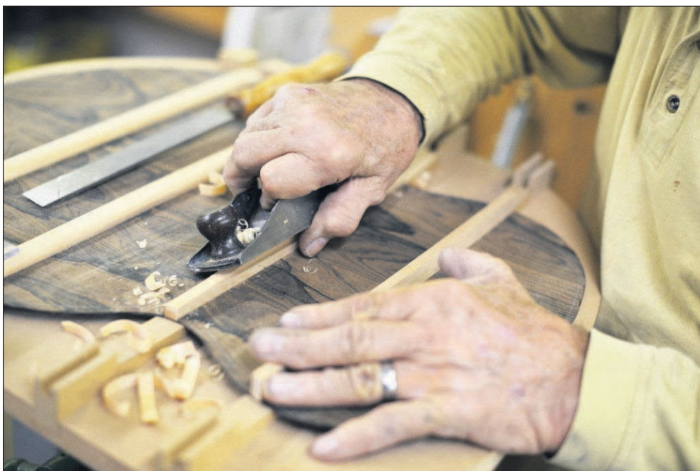
Left: Les McMasters uses a block planer to shape the braces on the back of a guitar at his shop in Hermiston. Right: Les McMasters inspects his craftsmanship while profiling the neck for a guitar using a spindle sander at his shop in Hermiston.
