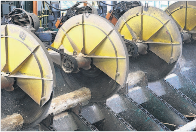
A multi-head radial saw cuts logs into blocks in the log utilization center at Boise Cascade's Elgin plywood mill.
