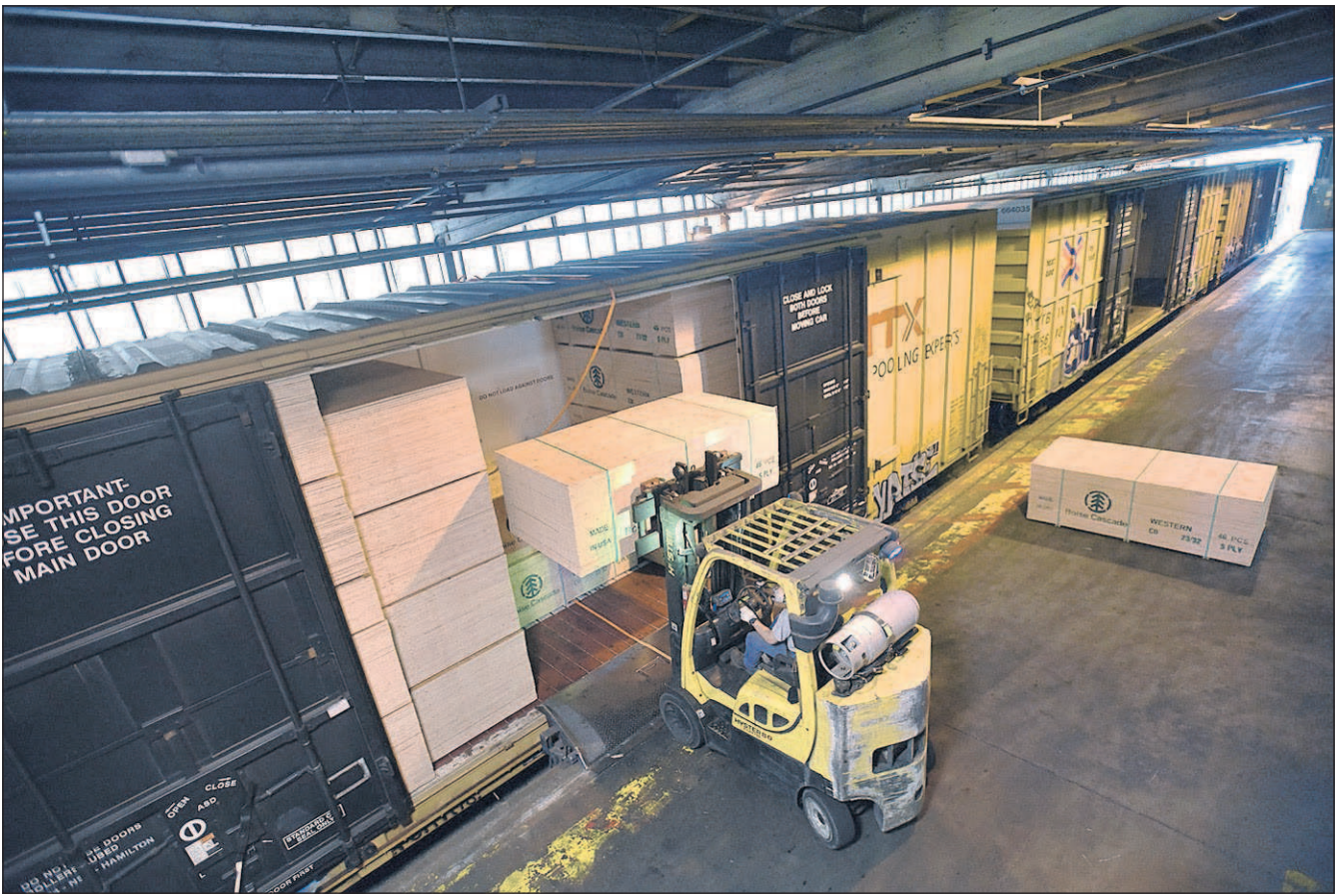
A forklift is used to load a pallet of plywood onto a railcar in the Boise Cascade Elgin plywood mill.
