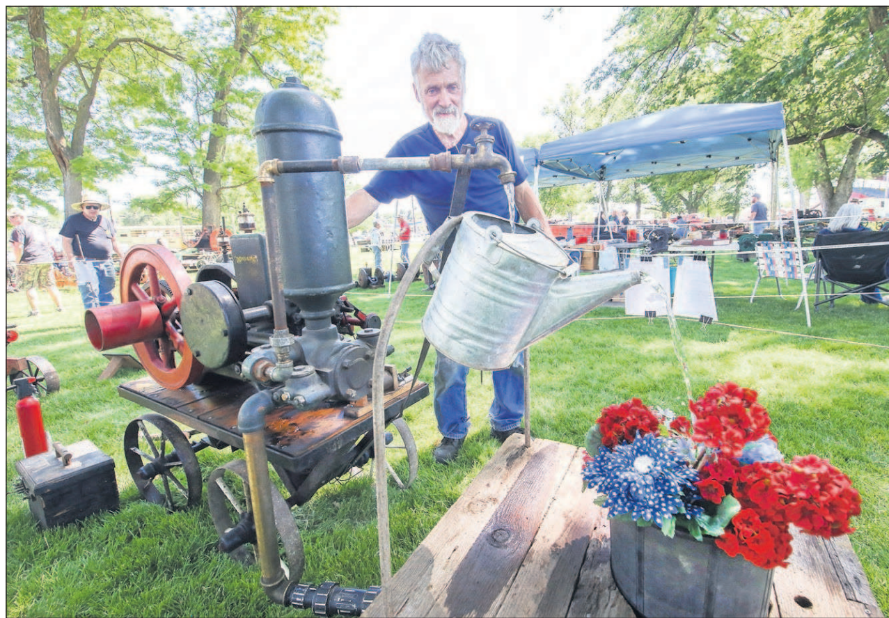
Dan Sudel, of Sherwood, demonstrates an old Domestic 1.5 horsepower engine he rigged to continually pump water to and from a flower arrangement at the Old Iron Show at Roy Raley Park. The exhibit, which features antique farm equipment, vintage cars, old engines and demonstration, runs through Sunday.
