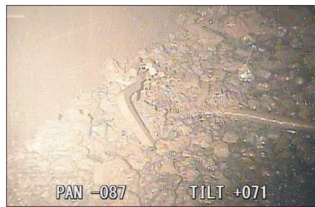
International Research Institute for Nuclear Decommissioning via AP A photo taken by a robotic probe shows a part of what is believed to be the handle of the fuel rods container and melted fuel in small lumps scattered on a structure below the Fukushima reactor core.
