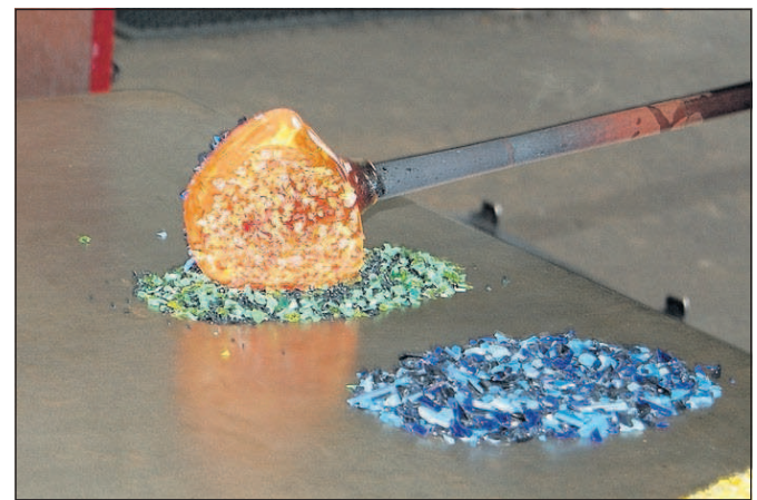
Crushed glass is added to molten glass that was heated to 2,100 degrees while creating a glass float at Jennifer Sears Glass Art Studio in Lincoln City. Staff photo by Tammy Malgesini
