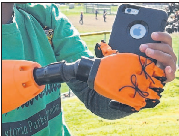
LEFT: Jude Rochon demonstrates how he can grasp items with his new 3D-printed prosthetic arm. Rochon can open and close the hand with the aid of a special harness he wears. RIGHT: Jude's mother, Alivia Rochon, helps adjust the prosthetic arm that works in conjunction with a harness that helps him control the hand.
