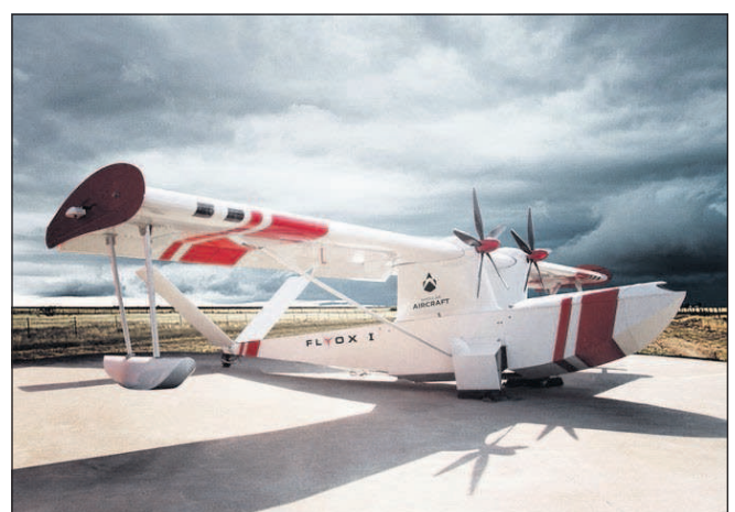
Photo contributed by Singular Aircraft The Flyox I has a maximum takeoff weight of 8,378 pounds with a 45-foot wingspan and 145 mph cruising speed. It is being developed to assist in firefighting.
