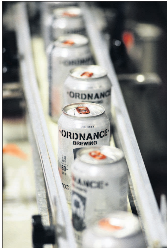
Topped and sealed cans of EOD Double IPA move down the production line during the canning process Thursday at Ordnance Brewing in Boardman. Staff photo by E.J. Harris
