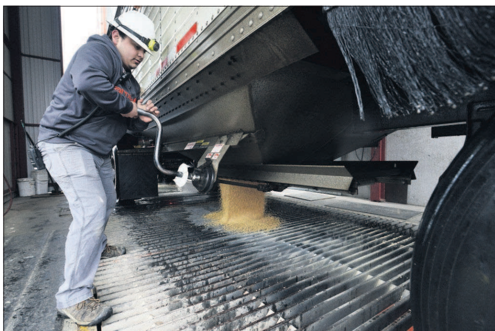
Wheat falls into a grate as operator Pete Veliz opens the bottom of a grain hopper at the United Grain McNary terminal on Monday in Umatilla.
