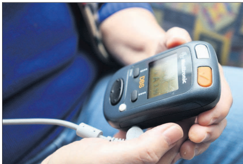
Carol Clupny, who recently underwent deep brain stimulation, holds a device called a patient programmer which allows her to control the neurostimulator embedded under her collarbone. With the programmer, Clupny can monitor battery life and control the current that flows into her brain within physician-prescribed limits.
