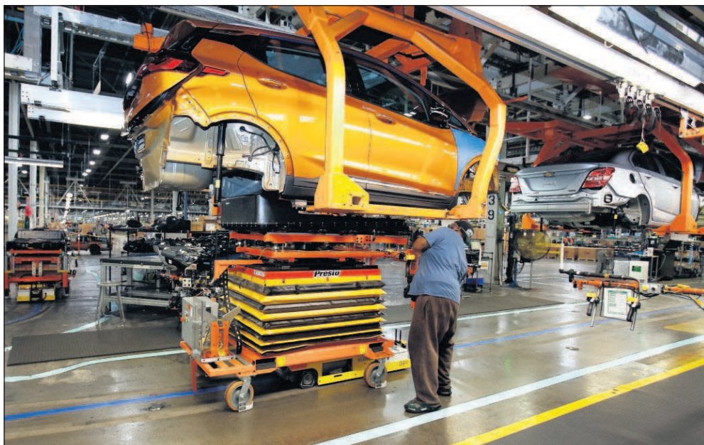
A battery is lifted into place for installation in the Chevrolet Bolt EV at the General Motors Orion Assembly plant Friday in Orion Township, Mich.
