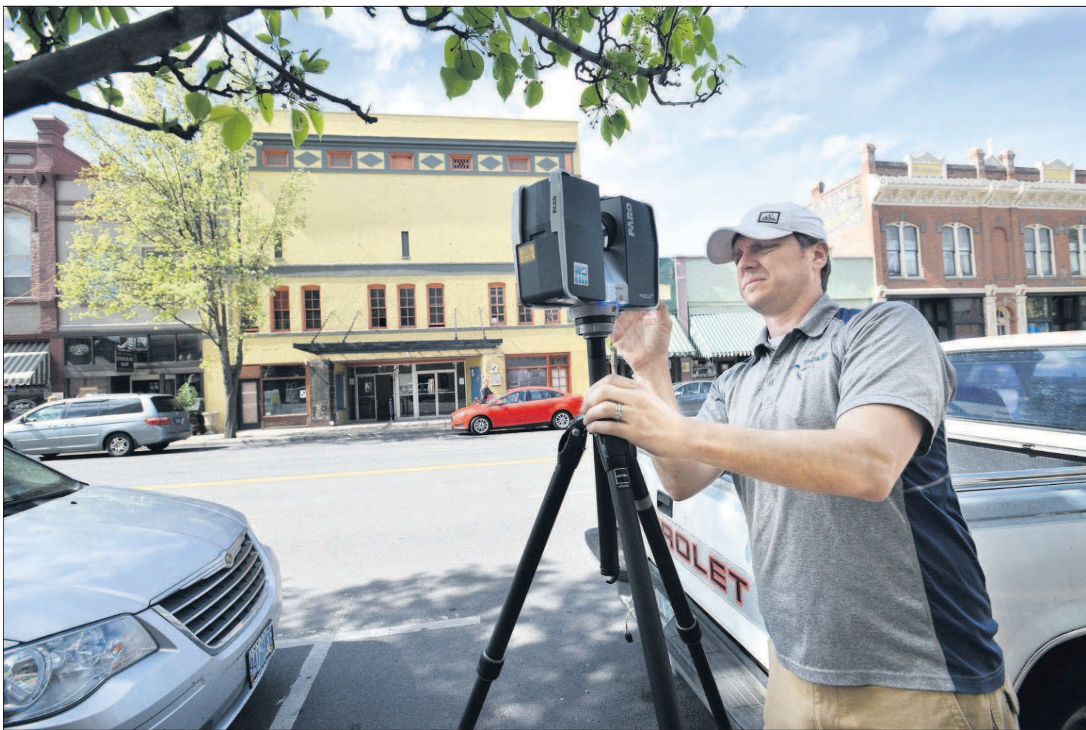
Staff photo by E.J. Harris Paul Tice, founder of ToPa 3D of Beaverton, sets up his 3D laser scanner outside of the Rivoli theater on Tuesday in Pendleton. Tice is using the scanner to create a 3D blueprint of the historic theater.
