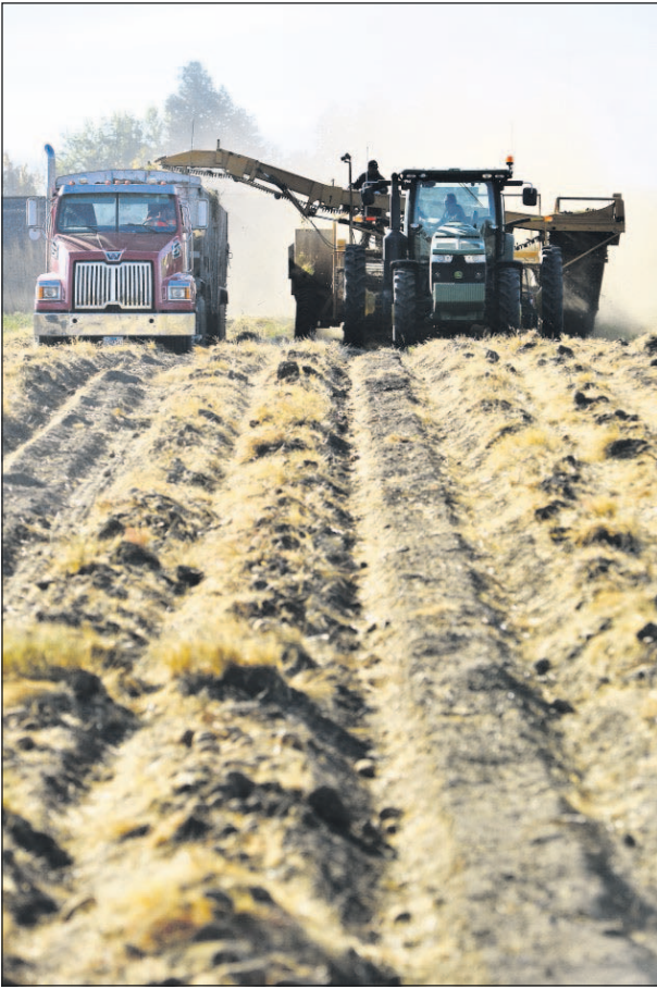
A potato harvester digs up and then loads potatoes into a semi trailer in a plot at the Hermiston Agricultural Research & Extension Center.
