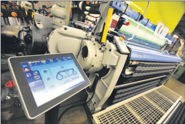
A touch screen control panel of the Pendleton Woolen Mills’ new Itema R9500 loom.
