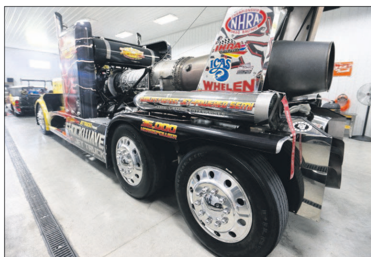
The semi-trailer known as Shockwave is parked in Springfield, Mo., June 8. The truck is powered by three jet engines producing 36,000 horse power.
