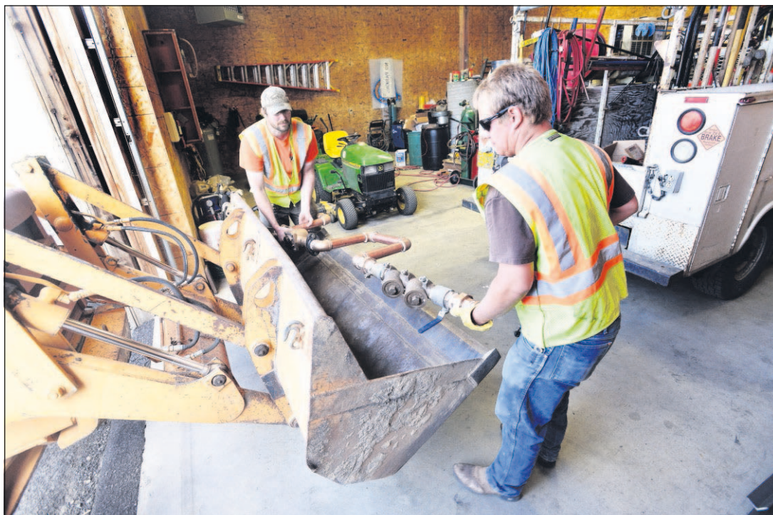
Curtis Thompson and Stewart Syverson, a temporary assistant to Thompson, lift a double check valve into a front-end loader at the Ione City Maintenance shop on Wednesday in Ione.
