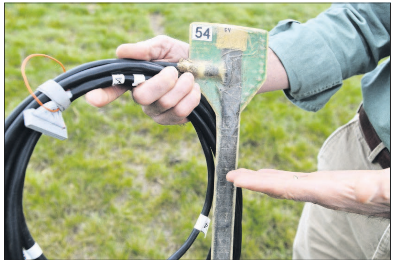
Soil scientist Stewart Wuest holds a thermometer he uses to measure soil temperatures below the surface of a crop. Staff photo by E.J. Harris
