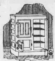
This refrigerator is seamless, porcelain lined, used in over a nillion and a half homes in America. The materials used in the Alaskan are seven walls of insulation, overhead circulation system, cors filled and equipped with removable, rost proof wire
