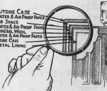
The insulation of a refrigerator is under the surface. It is the insulation, or lack of it, that determines the size of your ice bill.
