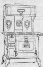
Twin flue construction enables you to heat all six lids on top of stove at an equal temperature without heating the oven. Saves heat in the room during summer months and saves fuel. Flue around oven is uniform in size so heated air comes in contact with every part of oven. We guarantee that pies or cakes can be baked even top and bottom and all sides without turning.
