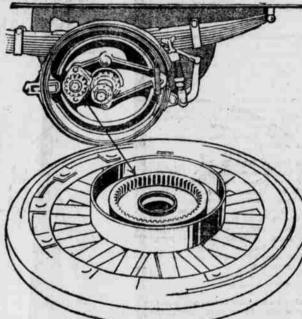
the internal gear drive—is the basis of several excel-lent makes of rear axle. The excellence of this form of power transmission is recognized almost universalby automotive engineers; and its widespread endorsement by truck users is evidenced by the pre-
