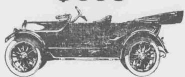
En bloc 35 horsepower motor. Electric starting and lighting
