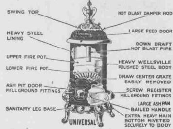
This cut shows the construction of the "Companion" Universal. Note the special features. Not new features with which we are experimenting but features that have made this Heater a reputation which cannot be denied.
