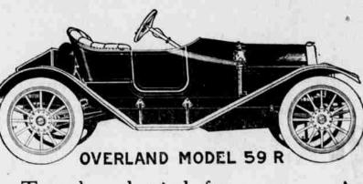
Tested and tried for years. FAVORITE wherever known. Each cylinder separate, 5 bearings to crank shaft, 3 point supension and genuine honeycomb radiator hung free as a wagon wheel.
