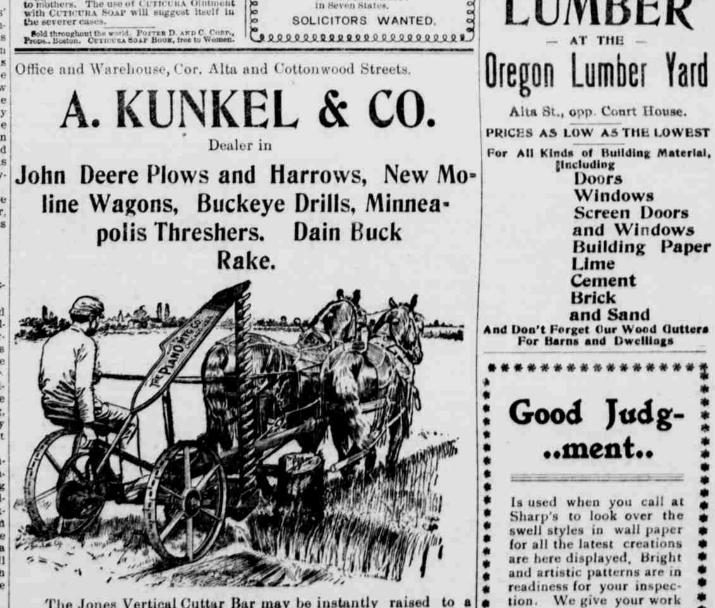
The Jones Vertical Cuttar Bar may be instantly raised to a vertical position, by the lifting levers while the machine is in motion; and the foot lift raises the bar much higher than any other machine, the sickle being thrown in and out of gear automatically.
