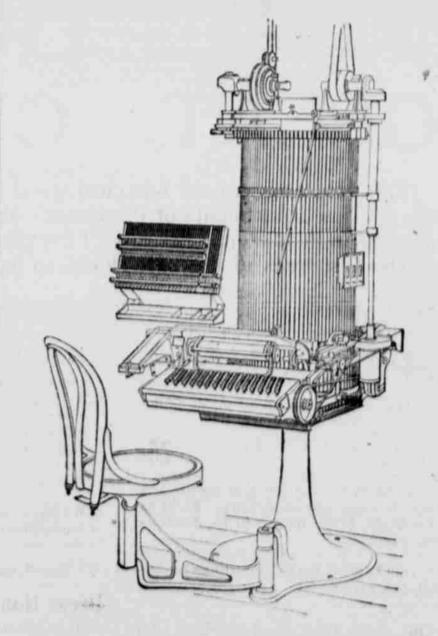
Machine is in good condition, requires only one quarter horse power to run it and with it one person can set from 20,000 to 25,000 ems brevier in eight hours.
