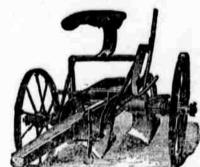
The greatest Labor-Saving Implements yet Invented. Vastly improved for Fall of 1877. 500 Sold in Oregon in One Year. EASILY OPERATED. So constructed that by a slight motion of the Lever the Plow is our out of the ground and raised clear, by horse-instead of man-power. It is stronger and
