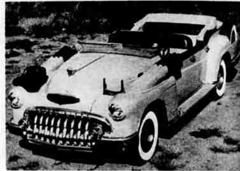
This Buick built for the King Ranch in Texas has wrangler's seat, gun holders, two-way telescope.
