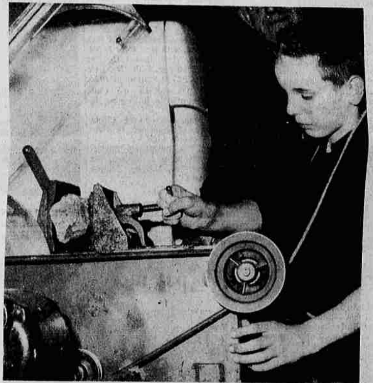
Joe Estes tightens vice on rock before adjusting plastic shatter-proof cover and starting motor on diamond saw.
