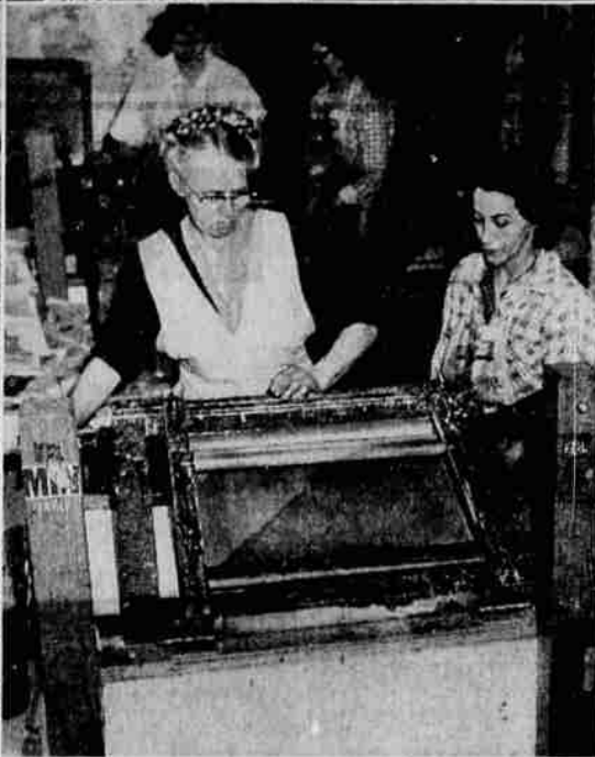
copy board. The line-drawing on the board will be copied for reduction. Lower left, Quintin Barton letters a decal. Barton does much of the original art work. And, lower right, Else Elgaard, left, and Marcella Davis do some silk screen printing. The sheets will be dried and then more color will be added. When the final clear coat is dried, the process is finished. This is another of Eugene's smaller industries.
