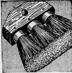
3-Knot Roof Brush Spreads Roof Paint Quickly
