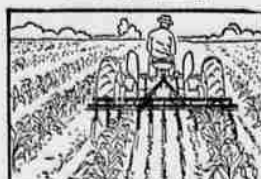
Hydraulic Touch Control sets sweeps or shovels for uniform working depth.
