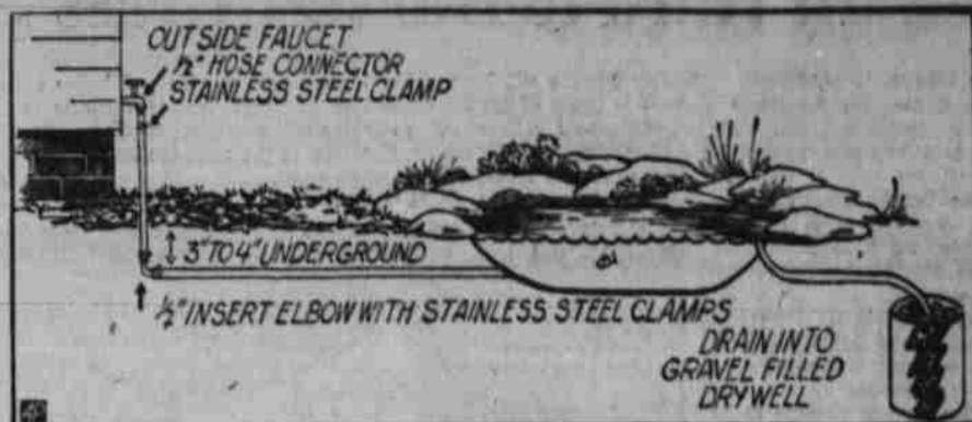
DIAGRAM for an easy-to-build goldfish pond, using plastic pipe.
