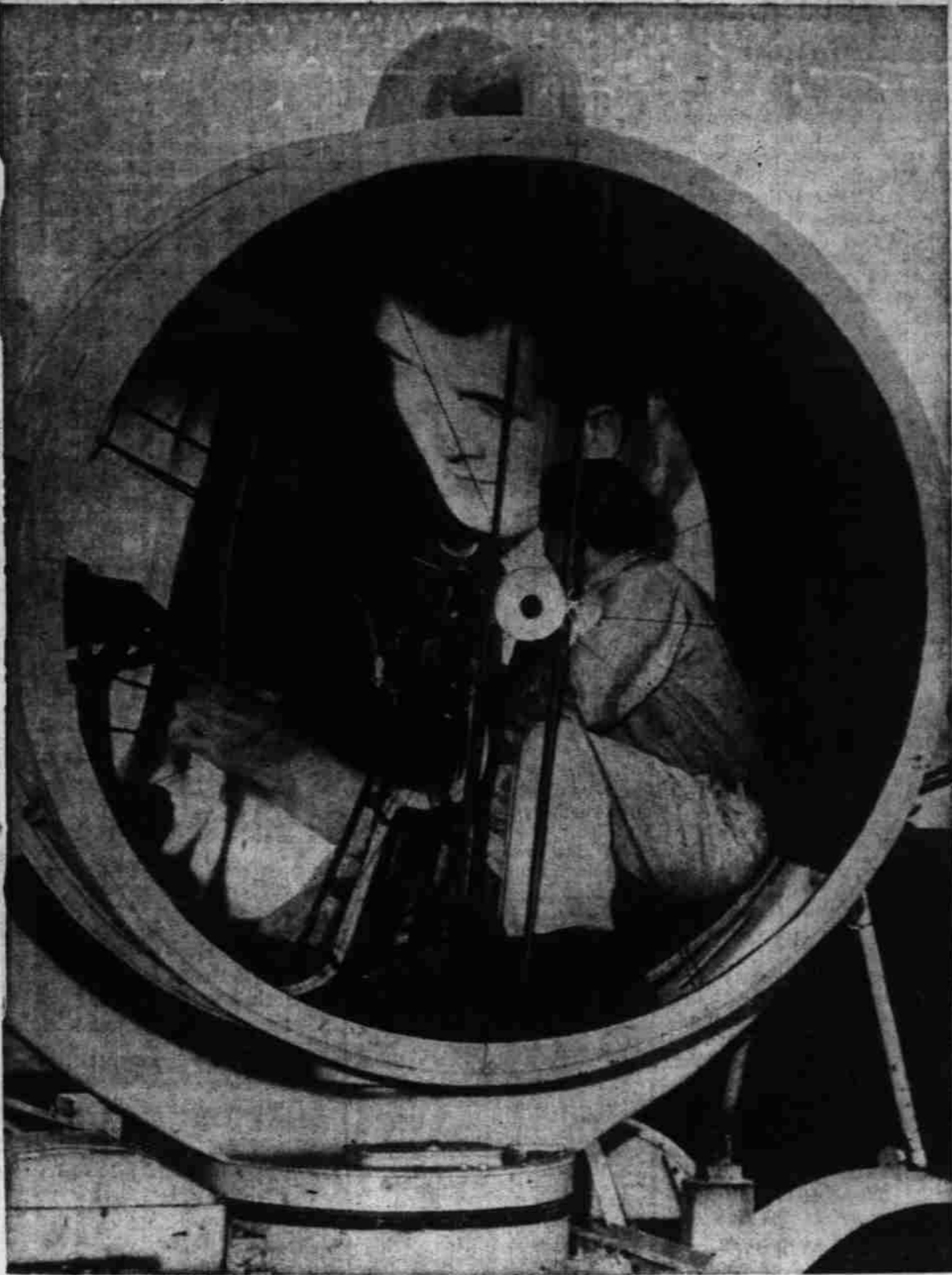
Cleaning a searchlight reflector is a big job, especially when the reflector is 60 inches high and the light weighs 350 pounds. Robert Wheeler, machinist at West Salem Machinery Co., is shown above polishing his magnified image in the shiny reflector on a large war-surplus arc light. The metal mirror shoots a beam of light 36,000 feet into the skies. (Statesman photo by John Erickson). (Story in sec. 1, page 4).
