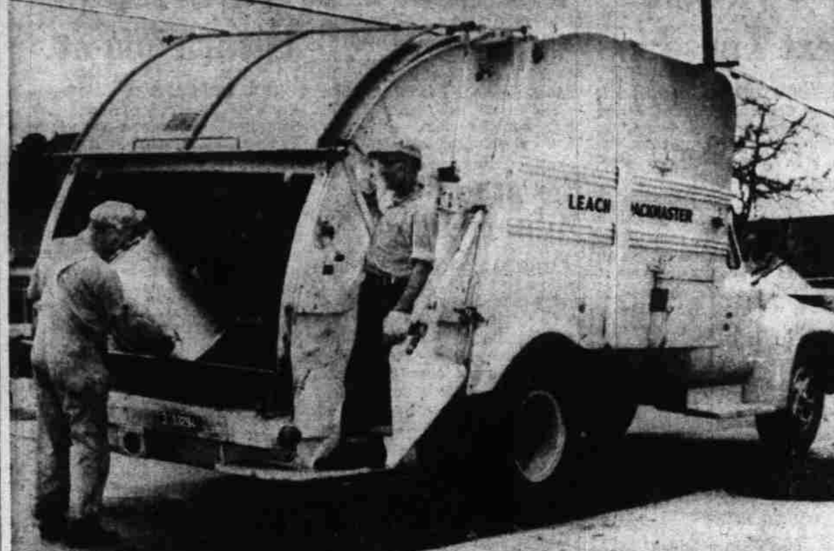
No climbing or boosting for these garbage collectors, shown above with one of Sanitary Service Company's newest trucks. Collector Hank Gugel, 3140 Jensen Ave., is shown dumping a load of refuse into the rear. From there an automatic scoop pulls the garbage into the truck's interior. Workman at right is Herman Haffner, 5075 Chehalis Ave. (Statesman photo)
