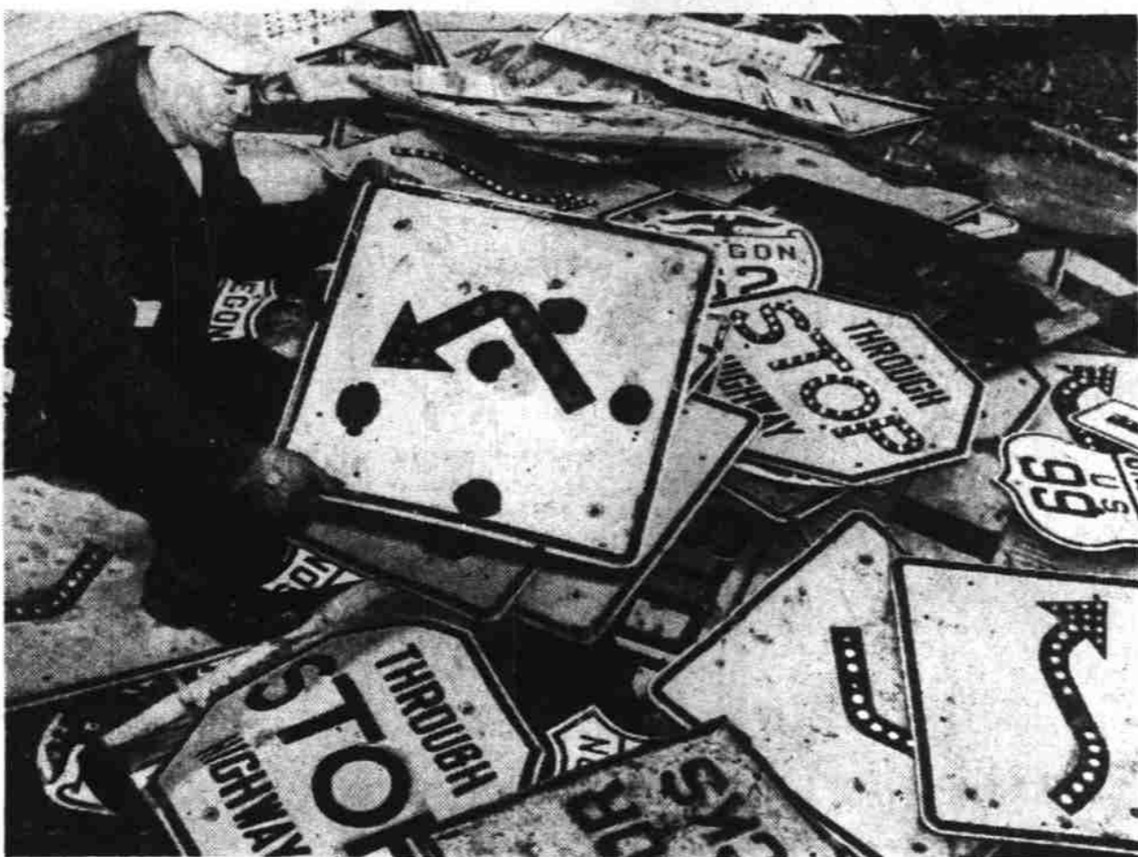
During hunting season, business at the state sign shops which is always good, gets even better. David Chilles, sign shop foreman is shown above holding one of the reasons for an increase in highway sign replacements—a sign punctured by bullets which cause the large rust spots shown. The rattled signs are being replaced by plywood signs which will not rust and are cheaper. (Statesman Photo.)
