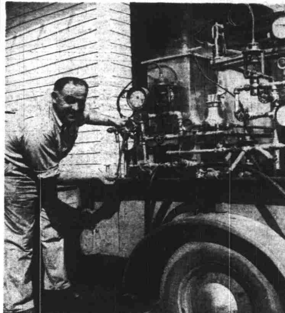
An 85-gallon portable pilot plant for peppermint oil distillation, built by A. D. Hughes, Oregon State College mechanical engineering professor, is pictured. Hughes takes this equipment to valley mint fields during harvest season and experiments in finding quicker, less expensive ways of distilling the oil from the peppermint hay.
