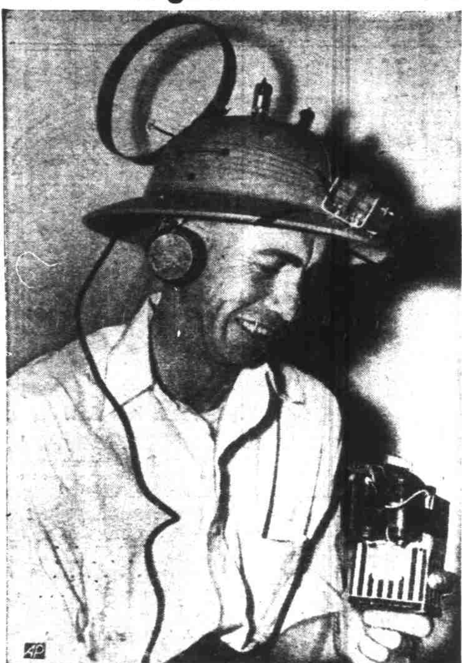
SPOKANE, Wash.—Look what Frank W. Elmore of Spokane, Wash., wears on his head—a hat radio. The dial is in front, tubes sticking up like horns on top and that circular thing is the aerial. A pocket battery, earphones and some other equipment inside the helmet do the rest. Just the thing for a gardener, says Elmore, an electrician. His hat tunes in all the local radio stations. (AP Wirephoto to The Statesman)
