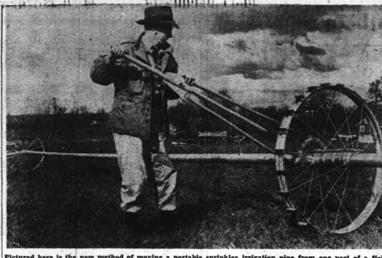
Pictured here is the new method of moving a portable sprinkler irrigation pipe from one part of a field to another. The new system has actually turned the conventional aluminum irrigation into one long axle for a series of specially designed wheels. With the aid of a ratchet drive, an entire one-eighth mile line of aluminum irrigation pipe can be rolled across a farm field by one man.
