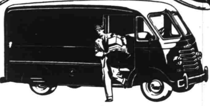
FORWARD-CONTROL CHASSIS Model 3742—125 1/4-inch wheelbase, Maximum G.V.W. 7000 lb. Also available in Model 3942—137-inch wheelbase, Maximum G.V.W. 10,000 lb. Package Delivery type Bodies suitable for mounting on the Forward-Control Chassis are supplied by many reputable manufacturers.
