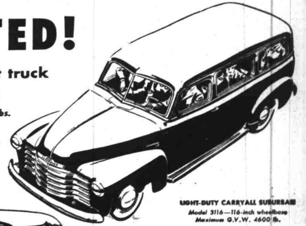
LIGHT-DUTY CARRYALL SUBURBAN Model 3116—116-inch wheelbase, Maximum G.V.W. 4600 lb.
